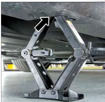
Front Jacking Location Engaged
