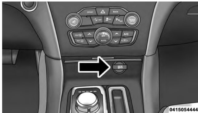
Front Power Outlet
