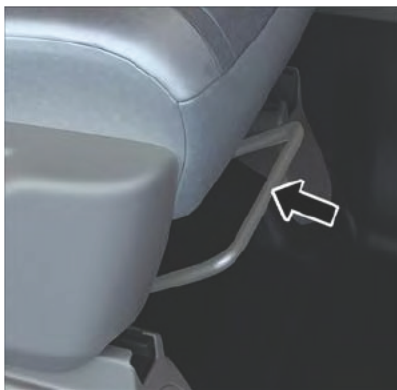
Adjusting Bar Location
