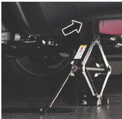
Front Jacking Location
