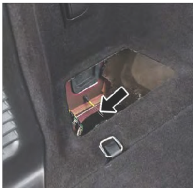
Emergency Release Cable
