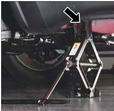
Front Jacking Location
