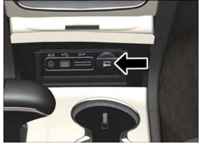
Front Power Outlet
