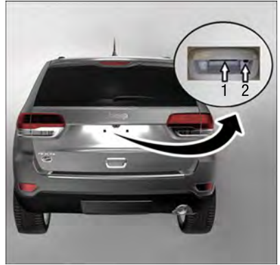
Electronic Release Switch Location
