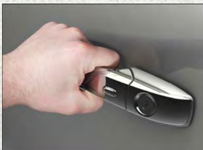
Grab The Door Handle To Unlock
