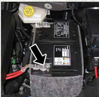
Positive Battery Post
