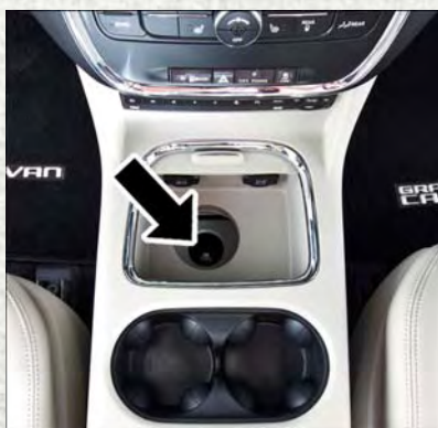
Winch Drive Nut Location
