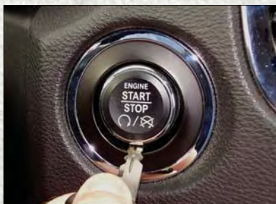
Removing START/STOP Button
