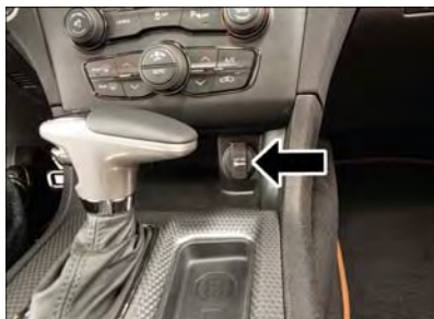
Front Power Outlet
