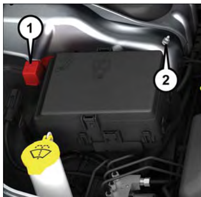
Remote Battery Posts
