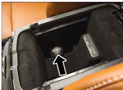
Center Console Power Outlet
