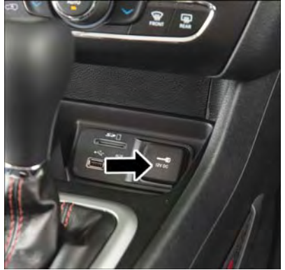
Front Power Outlet
