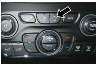
STOP/START OFF Switch
