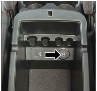
Center Console Power Outlet
