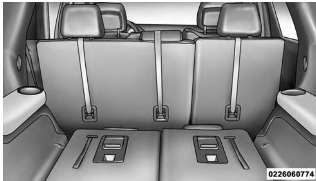
Top Tether Strap Mounting (60/40 Seat)
