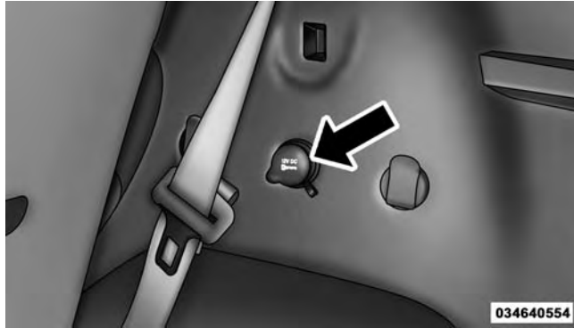
Rear Cargo Power Outlet
