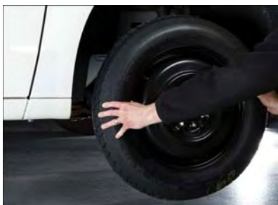
Installing Compact Spare
