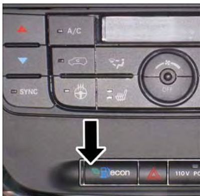
ECON Switch Location
