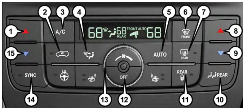
Three Zone Automatic Temperature Controls (ATC)
