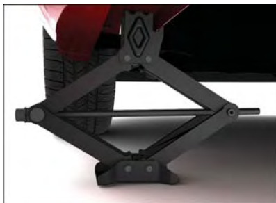
Rear Jacking Location Engaged
