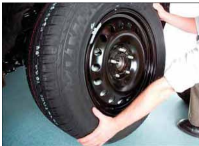
Installing Spare Wheel/Tire
