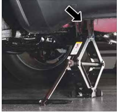
Front Jacking Location
