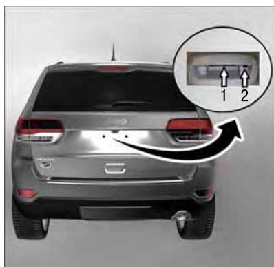
Electronic Release Switch Location
