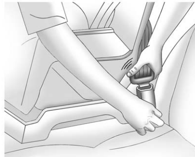
Tilt the latch plate to adjust the belt, if needed.
