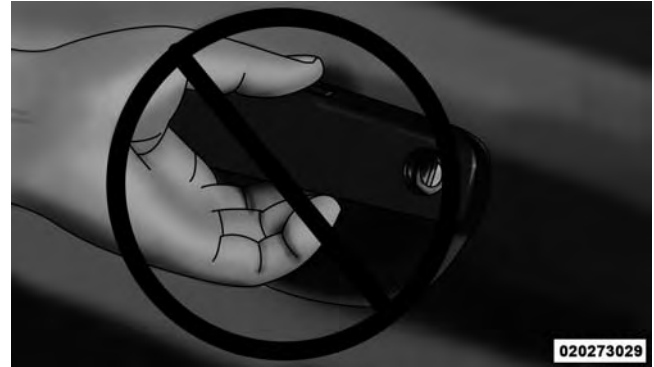
Do NOT Grab The Handle When Locking
