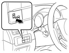
When the Blind Spot Monitoring (BSM) switch is pressed, the Blind Spot Monitoring (BSM) and Rear Cross Traffic Alert (RCTA) systems are turned off and the Blind Spot Monitoring (BSM) OFF indication/indicator light in the instrument cluster turns on.
