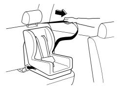
5. Push the child-restraint system firmly into the vehicle seat. Be sure the belt retracts as snugly as possible. A clicking noise from the retractor will be heard during retraction if the system is in the automatic locking mode. If the belt does not lock the seat down tight, repeat this step.
