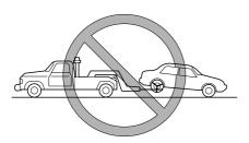
Do not tow with sling-type equipment. This could damage your vehicle. Use wheel-lift or flatbed equipment.
