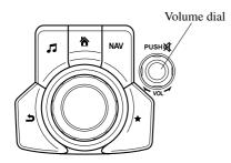
Press the volume dial to switch the audio MUTE on and off. Turn the volume dial to adjust the volume. The volume increases by turning the dial clockwise, and decreases by turning it counterclockwise.
