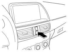
Depress the hazard warning flasher switch and all the turn signals will flash. The hazard warning indicator lights in the instrument cluster flash simultaneously.
