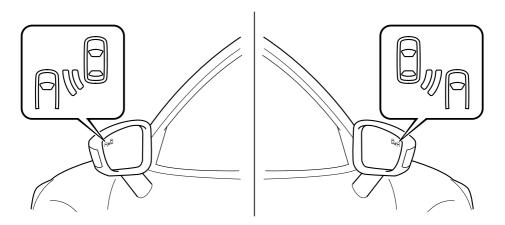
When the ignition is switched ON, the malfunction warning light turns on momentarily and then turns off after a few seconds.
