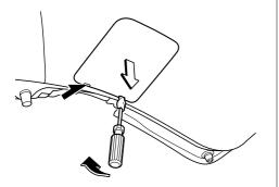
3. Turn the socket and bulb assembly counterclockwise and remove it.
