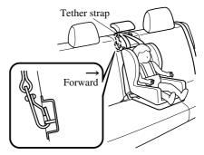
Always attach the tether strap to the correct tether anchor position:
