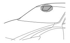
The Forward Sensing Camera (FSC) determines the conditions ahead of the vehicle while traveling at night and detects traffic lanes. The distance in which the Forward Sensing Camera (FSC) can detect objects varies depending on the surrounding conditions.
