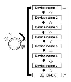
5. Press the audio control dial to select the device you would like to link. The ♪ symbol disappears, and "PAIRING" flashes in the audio display.
