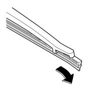
4. Remove the metal stiffeners from the blade rubber and install them in the new blade.
