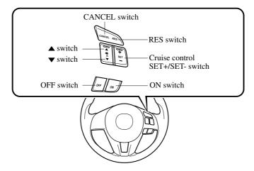
When the ON switch is pressed, the vehicle speed and the distance between vehicles while in headway control can be set. The Mazda Radar Cruise Control (MRCC) indication is shown in the display of the instrument cluster.
