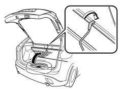
3. Turn the spare tire hold-down bolt counterclockwise.
