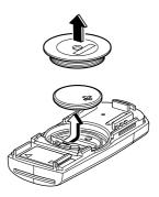
6. Insert a new battery with the positive pole facing up, and then cover the battery with the battery cap.
