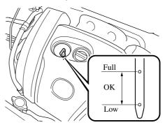
Pull it out again and examine the level. The level is normal if it is between Low and Full. If it is near or below Low, add enough
