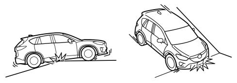
Your vehicle is equipped with low profile tires allowing class-leading performance and handling. As a result, the sidewall of the tires are very thin and the tires and wheels can be damaged if driven through potholes or on rough/uneven roads at excessive speeds. Use care and reduce speed when traveling on rough/uneven roads or through potholes.
