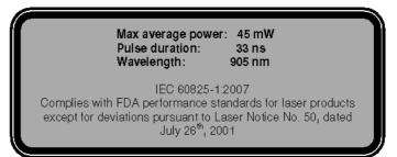
Laser sensor radiation data Maximum average power:45 mW Pulse duration:33 ns Wavelength:905 nm Divergence angle (horizontal×vertical):28 degrees×12 degrees
