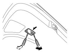
2. Disconnect the electrical connector from the bulb by pressing the tab on the connector with your finger and pulling the connector.
