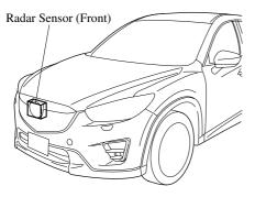
If "Front radar blocked" is displayed in the multi-information display of the instrument cluster, clean the area around the radar sensor (front).
