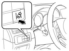
On the type A instrument cluster, the lane indication (border line) is indicated in the multi-information display. **Indication on display**
