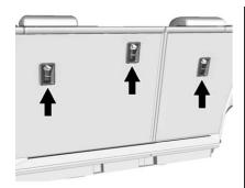
The top tether anchors are on the back of the rear seatbacks. Be sure to use an anchor on the same side of the vehicle as the seating position where the child restraint will be placed.
