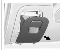
The instrument panel fuse block is on the underside of the driver side instrument panel. To access the fuses, remove the storage compartment. To remove the storage compartment, open the compartment and pull it out.
