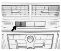
The button for TCS and StabiliTrak is on the center stack.
