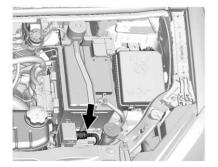
Open the hood and unwrap the electrical cord. The cord is located in the driver side of the engine compartment, near the battery. It is shipped from the factory with a tie holding it in place. Use care in removing the tie so that the cord is not damaged.
