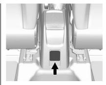
An indicator light on the outlet turns on to show it is in use. The light comes on when the ignition is in ON/RUN and equipment requiring less than 150 watts is plugged into the outlet, and no system fault is detected.
