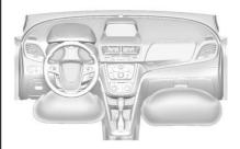
The driver knee airbag (if equipped) is below the steering column. The front outboard passenger knee airbag (if equipped) is below the glove box.
