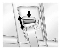
To move the shoulder belt height adjuster down, push down on the release button and move the height adjuster to the desired position. You can move the height adjuster up by pushing up on the shoulder belt quide.
