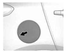
The fuel cap is behind a hinged fuel door on the right rear side of the vehicle.
