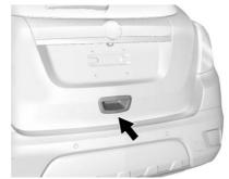
To open the liftgate, press the touch pad in the pull cup under the license plate and lift manually.
