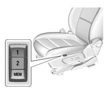
If available, the MEM, 1, and 2 buttons on the outboard side of the driver seat are used to manually store and recall the driver seat and
