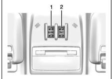
If equipped, the sunroof only operates when the ignition is turned to ON/RUN or Retained Accessory Power (RAP) is active.
