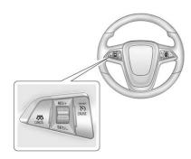
CRUSE (On/Off): Press to turn the cruise control system on or off. A white indicator comes in the instrument cluster when cruise is turned on.
