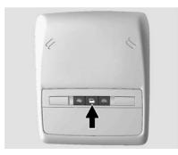
The front dome lamp controls are in the overhead console.
