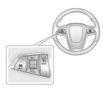
CRUST : Press to turn the cruise control system on or off. A white indicator comes in the instrument cluster when cruise is turned on.
