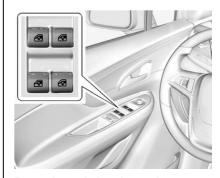
Press the switch to lower the window. Pull up on the front edge of the switch to raise it. See *Power Windows* ⇔ 37.
