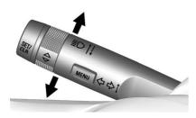
(Headlamp High/Low-Beam Changer): Push the turn signal lever away from you and release, to turn the high beams on.
