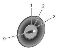
The ignition switch has four different positions.
