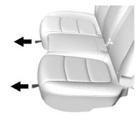
Pull the strap on the front edge of the rear seat cushion to release the cushion. Tilt the seat cushion forward toward the front of the vehicle. The seat cushion must be tilted forward before the seatback is folded down. Otherwise, the seatback will not fold down properly.
