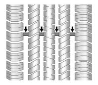
Treadwear indicators are one way to tell when it is time for new tires. Treadwear indicators appear when the tires have only 1.6 mm (1/16 in) or less of tread remaining. See *Tire Inspection* ⋄ 235 and *Tire Rotation* ⋄ 235.
