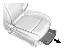
If equipped, there is storage under the front passenger seat. Lift the end of the tray and pull it forward to open. Push it in toward the seat to close.
