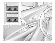
The driver door also has switches that control the passenger and rear windows. The switches work when the vehicle is in ON/RUN or ACC/ ACCESSORY, or when Retained Accessory Power (RAP) is active. See Retained Accessory Power (RAP)
