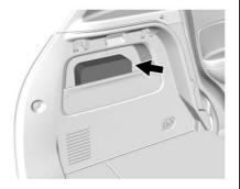
If equipped, the first aid kit is stowed in the side rear storage compartment.
