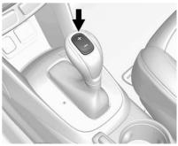
DSC allows you to shift an automatic transmission similar to a manual transmission. To use the DSC feature:
