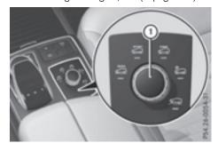
► All vehicles (except Mercedes-AMG vehicles): turn DYNAMIC SELECT controller ① as many times as necessary until the desired drive program is selected.
