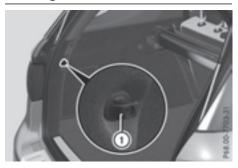
There is one securing hook (1) on each side of the cargo compartment.
