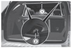
▶ Pull the cargo net up by tab (1) and hook it into eyelets (2) using both hands.
