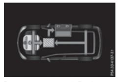
The engine powers the vehicle. The electric motor is operating as a generator, e.g. in overrun mode and when braking (▷ page 253). The kinetic energy of the vehicle is converted into electrical energy. The high-voltage battery is being charged.
