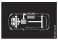
The engine powers the vehicle. If the vehicle is approaching a downhill gradient with a high potential for energy recuperation, the condition of charge of the high-voltage battery is intentionally kept low or intentionally reduced.
