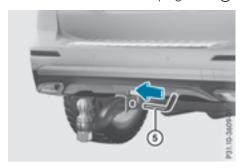
► Slide bolt ⑤ into the hole in the ball coupling recess and the ball coupling to the stop.
