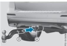
▶ Insert the ball coupling horizontally into ball coupling recess ② in the direction of the arrow until the holes in ball coupling ③ are in line with the holes in ball coupling recess ④.
