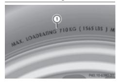
Maximum tire load ① is the maximum permissible weight for which the tire is approved. Do not overload the tires by exceeding the specified load limit. The maximum permissible load can be found on the vehicle's Tire and Loading Information placard on the B-pillar on the driver's side (> page 397).
