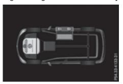
The combustion engine is running while the vehicle is stationary. The high-voltage battery is not being charged.
