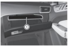
Partition (1) for stowing flat objects is located in the upper section of the glove box. It can be removed to increase the stowage space in the glove box.
