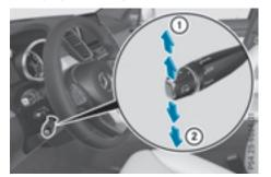
➤ To increase or reduce the set speed in 1 mph increments (Canada: 1 km/h increments): briefly press the cruise control lever up ① for a higher set speed or down ② for a lower set speed.
