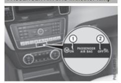
PASSENGER AIR BAG ON indicator lamp ① and PASSENGER AIR BAG OFF indicator lamp ② are part of the Occupant Classification System (OCS).
