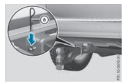
▶ Secure the bolt using spring cotter (6).
