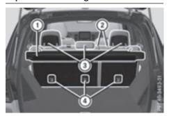
Top Tether anchorage points (4) are located on the rear side of the rear seat backrests.
