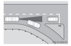
DISTRONIC PLUS does not brake for obstacles or stationary vehicles. If, for example, the detected vehicle turns a corner and reveals an obsta-
