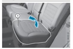
If the driver's or front-passenger seat is set for a larger person, it may not be possible to fold the rear bench seat forward. In this case, move the front seats as far forward as possible.
