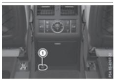
Vehicles with the Rear Seat Entertainment System have two sockets in the center console in the rear compartment.
