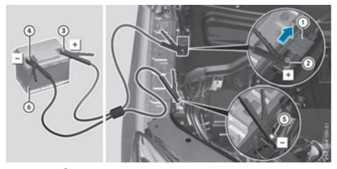
$Position \ number \ \textcircled{\scriptsize 6} \ identifies \ the \ charged \ battery \ of \ the \ other \ vehicle \ or \ an \ equivalent \ jump-starting \ device.$
