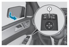
If you have switched the Auto. Mirror Folding on and you fold the exterior mirrors in using button ①, they will not fold out automatically (> page 111).
