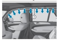
Window curtain air bags (1) are integrated into the side of the roof frame and deployed in the area from the A-pillar to the C-pillar.
