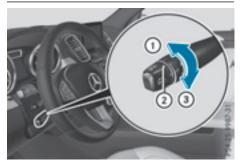
You can set the specified minimum distance for DISTRONIC PLUS by varying the time span between one and two seconds. With this function, you can set the minimum distance that DISTRONIC PLUS keeps to the vehicle in front, dependent on vehicle speed. You can see this distance in the multifunction display (> page 198).
