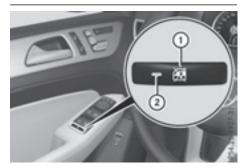
▶ To activate/deactivate: press button (1). If indicator lamp (2) is lit, operation of the rear side windows is disabled. Operation is only possible using the switches in the driver's door. If indicator lamp (2) is off, operation is possible using the switches in the rear compartment.
