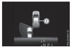
If a course-correcting brake application occurs, red warning lamp (1) flashes in the exterior mirror and a dual warning tone sounds. In addition, display (2) underlining the danger of a side collision appears in the multifunction display.
