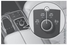
➤ Turn DYNAMIC SELECT controller ① as many times as necessary until the desired drive program is selected.
