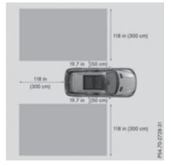
Blind Spot Assist monitors the area up to 10 ft (3 m) behind your vehicle and directly next to your vehicle, as shown in the diagram.
