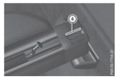
▶ Make sure that the red lock verification indicator (4) is no longer visible. The combined cargo cover and net will otherwise not be locked in place.
