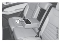
Fold down the rear seat armrest. Cup holder (1) is located in the rear seat armrest.
