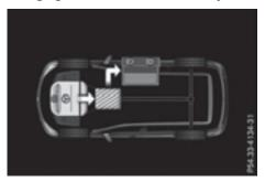
The engine powers the electric motor. The electric motor operates as a generator. The high-voltage battery is being charged.
