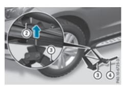
▶ Position jack (3) at jacking point (2). The alignment bolt on the jack must be inserted into the intended opening on the jacking point.
