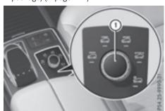
► Mercedes-AMG vehicles: turn DYNAMIC SELECT controller ① as many times as necessary until the desired drive program is selected.
