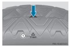
Marking (1) shows where the bar indicator (arrow) for tread wear is integrated into the tire
