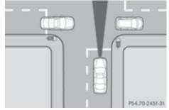
DISTRONIC PLUS may mistakenly detect vehicles that are crossing your lane. Activating DISTRONIC PLUS at traffic lights with crossing traffic, for example, could cause your vehicle to pull away unintentionally.
