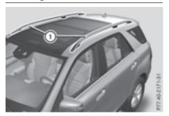
► Secure the roof carrier to roof rails ①. In doing so, observe the manufacturer's installation instructions.
