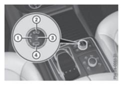
Set the vehicle level using the selector wheel.
