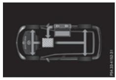
The electric motor powers the vehicle. The high-voltage battery supplies energy to the electric motor.
