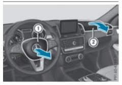
Driver's air bag (1) deploys in front of the steering wheel. Front-passenger front air bag (2) deploys in front of and above the glove box. When deployed, the front air bags offer additional head and thorax protection for the occupants in the front seats.
