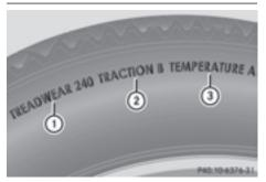
Uniform Tire Quality Grading Standards are U.S. government specifications. Their purpose is to provide drivers with uniform reliable information on tire performance data. Tire manufacturers have to grade tires using three performance factors: ① tread wear grade, ② traction grade and ③ temperature grade. These regulations do not apply to Canada. Nevertheless, all tires sold in North America are provided with the corresponding quality grading markings on the sidewall of the tire.
