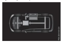
The electric motor is operating as a generator, e.g. in overrun mode and when braking. The kinetic energy of the vehicle is converted into electrical energy. The high-voltage battery is being charged.
