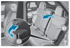
You can adjust the angle of the backrests in the second row of seats. There are several possible detent positions.
