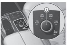
The very firm setting of the suspension setting in the **Sport Plus** drive program ensures the best possible contact with the road. Select this drive program when employing a sporty driving style, e.g. on winding country roads or primarily when driving on race circuits.
