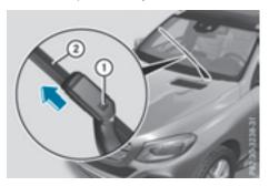
► Firmly press release knob ① and pull wiper blade ② upwards from the wiper arm in the direction of the arrow.
