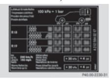
Some tire pressure tables show only the rim diameters instead of the full tire size, e.g. **R18**. The rim diameter is part of the tire size and can be found on the tire sidewall (> page 403).
