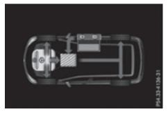
If you accelerate the vehicle rapidly, the electric motor supports the combustion engine by providing additional drive torque.
