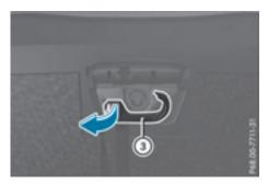
► Fold out hook (3) on the underside of the cargo compartment floor in the direction of the arrow.
