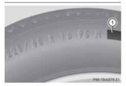
In addition to the load bearing index, load index 1 may be imprinted after the letters that identify speed index 6 on the sidewall of the tire ( $\triangleright$  page 403).
