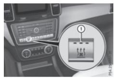
➤ To activate or deactivate "Immediate preentry climate control": press button ①. The blue or red indicator lamp in the button lights up or goes out.
