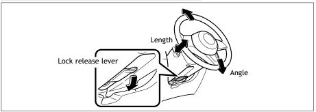
Hold wheel, push lever down, set angle and return lever.
