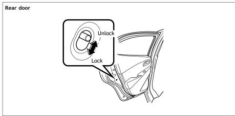
Moving the lever downward will allow the door to be opened only from the outside.
