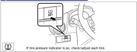
After adjusting tire pressures, or after tires have been rotated or replaced, turn the ignition switch to "ON" and press and hold the "-SET" button until indicator blinks twice and a beep sound once. Let the vehicle sit for a few minutes to allow initialization to complete.
