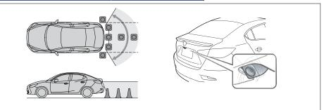
The rear view monitor system displays an image of the view from the bumper of the rear area of the vehicle. The camera for the rear view monitor system is located above the license plate.
