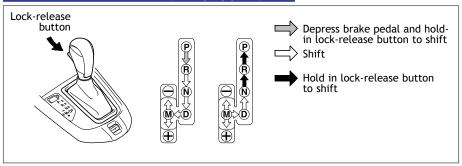
The ignition switch must be "ON."
