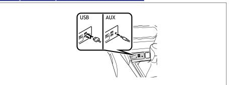
Ignition switch must be in the "ACC" or "ON" position to use. Use these ports to connect a portable audio device and listen to it through the vehicle's speakers.
