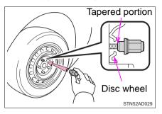
Tighten the nuts until the tapered portion comes into loose contact with the disc wheel.
