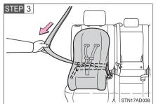
Fully extend the shoulder belt and then allow it to retract slightly in order to activate the ALR lock mode.
