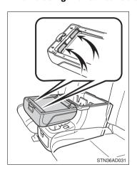
Close the rear console box by lifting the grip on the inside of the upper box.
