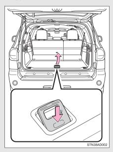
Pull the lever upwards to lift the deck board.
