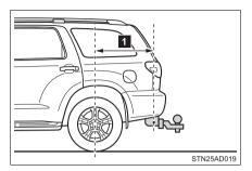
■ Hitch receiver pin hole position: 46.2 in. (1172.3 mm)
