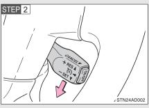
Accelerate or decelerate the vehicle to the desired speed, and push the lever down to set the speed.
