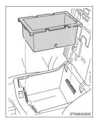
The box can be removed. Hanging file folders can be hung on the rails when the box is removed.
