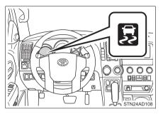
The slip indicator will flash while the VSC/Trailer Sway Control/TRAC/ A-TRAC systems are operating.
