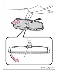
Hold and rotate the mirror to adjust the support.
