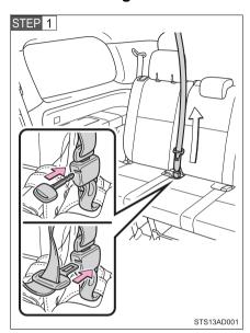
To release the hooked end tab, insert the key or concaved end tab into the hole on the buckle.
