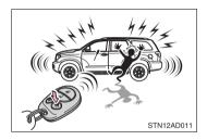
When sout one second, an alarm will sound for about 60 seconds and the vehicle lights will flash to deter any person from trying to break into or damage your vehicle.
