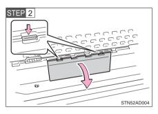
Remove the cover and loosen the strap.
