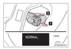
1 Press the ON-OFF button to activate the cruise control.
