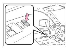
Press the switch down to lock passenger window switches and back window switch.
