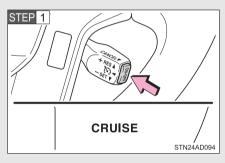
Press the ON-OFF button to activate the cruise control.
