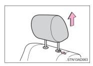
Pull the head restraint up while pushing the lock release button.
