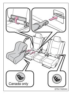
Latch the hooks of the lower straps onto the LATCH anchors and tighten the lower straps.
