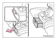
Pull the lever up to release the lock. Pull the handle.
