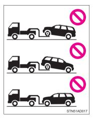
2WD models: Be sure to transport the vehicle with all four wheels raised off the ground. If the vehicle is towed with the tires contacting the ground, the drivetrain and related parts may be damaged or an accident may occur due to a change in direction of the vehicle.
