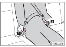
Make sure that the buckle **1** is securely latched for ready use of the center seat belt.
