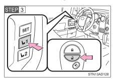
Push the "1" or "2" button and the putton on the wireless remote control at the same time for about 1 second until you hear a beep.
