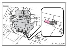
Depress the release pedal and fold down the seatback. The seat will slide forward.
