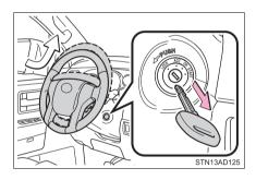
When the key is removed from the engine switch, the steering wheel returns to its stowed position by moving up and away to enable easier driver entry and exit.
