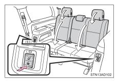
Press and hold the seatback folding switch until the seatback folds down fully and the buzzer sounds
