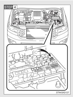
Remove the fuse with the pullout tool.
