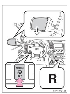
Press the switch to turn on/off linked mirror function.
