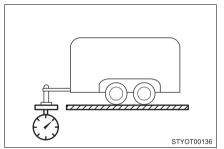
The load placed on the trailer hitch ball. ( $\rightarrow$ P. 276)
