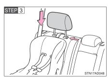
Latch the hook onto the anchor bracket and tighten the top tether strap.
