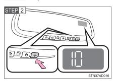
Press the switch until a number (1 to 15) appears on the compass display.
