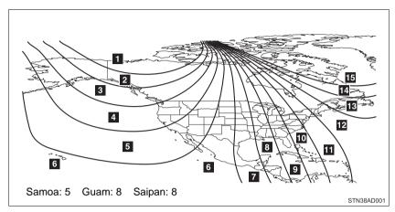
The direction display deviates from the true direction determined by the earth's magnetic field. The amount of deviation varies according to the geographic position of the vehicle.
