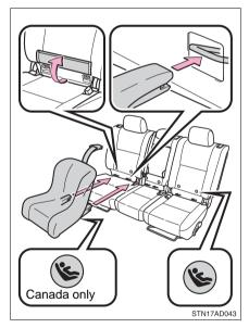
Fold the seatback while pulling the lever. Return the seatback and secure it at the 1st lock position (most upright position). Adjust the seatback to the 8th lock position. (→P. 51)
