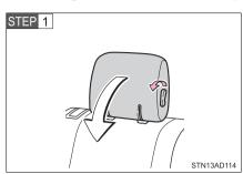
Pull the head restraint lock release lever to fold the head restraint.
