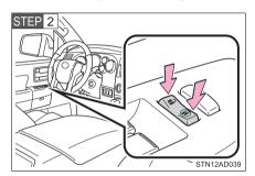
Shift the shift lever to P or N, press and hold the driver's door lock switch ( or or approximately 5 seconds and then release.
