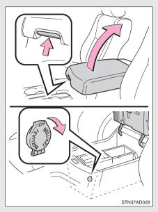
Pull the knob up to release the lock. Lift the lid.
