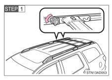
Turn the knobs counterclockwise to loosen the cross rails.
