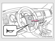
To sound the horn, press on or close to the mark.
