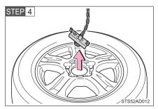
After the tire is lowered completely to the ground, remove the holding bracket.
