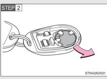
Remove the discharged transmitter battery.
