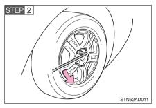
Slightly loosen the wheel nuts (one turn).
