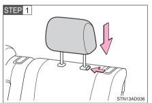
Adjust the head restraint to the downmost position.
