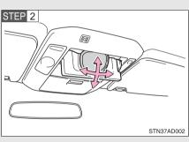
The mirror can be adjusted by pushing the mirror edge.
