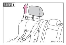
Secure the child restraint using the LATCH anchors or seat belt, and adjust the head restraint to the upmost position.
