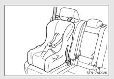
Seat belts equipped with a child restraint locking mechanism (ALR/ELR belts except driver's seat belt) (→P. 69)
