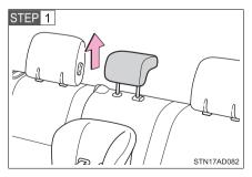
Secure the child restraint using the LATCH anchors or seat belt, and adjust the head restraint to the upmost position.
