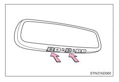
Press and hold down the 2 outside buttons for 10 seconds until the indicator flashes.
