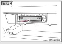
Pull the filter out of the filter outlet.
