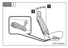
Fold the seatback while pulling the lever. Return the seatback and secure it at the 1st lock position (most upright position). Adjust the seatback to the 4th lock position. (→P. 51)
