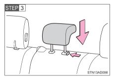
Adjust the center head restraint to the downmost position.
