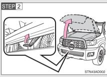
Pull up the hood catch lever and lift the hood
