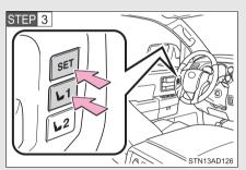
While pushing the SET button, push button "1" or "2" until the signal beeps.
