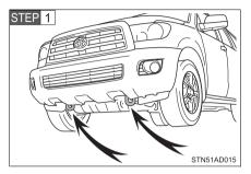
Securely attach cables or chains to the towing hooks.
