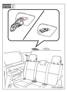
Stow the seat belt tabs in the cover set in the roof as shown.
