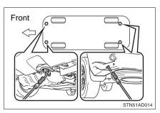
If your vehicle is transported by a flatbed truck, it should be tied down at the locations shown in the illustration.
