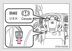
the Set parking brake\*. (Depressing the pedal again releases the parking brake.)
