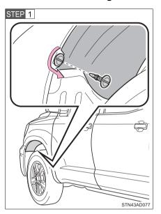
Remove the fender liner clip.
