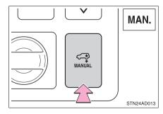
When the height control mode select switch is pressed, the vehicle height is fixed at the current height.
