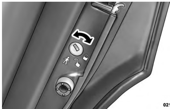
Child-Protection Door Lock Function
