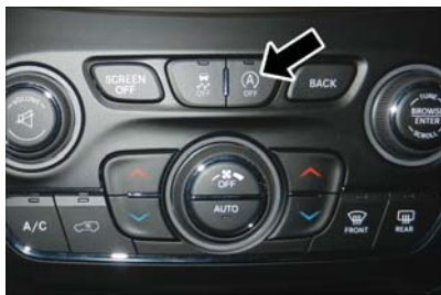
STOP/START OFF Switch
