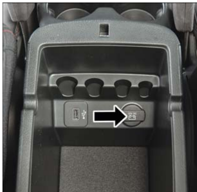
Center Console Power Outlet
