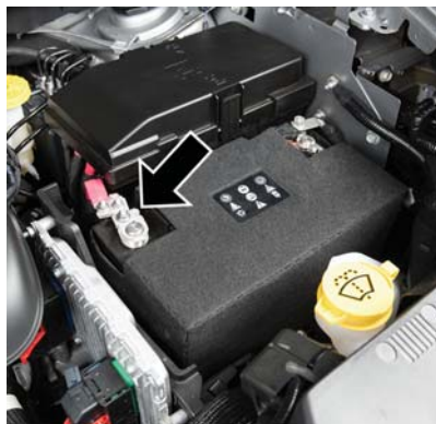
Positive Battery Post
