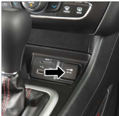
Front Power Outlet
