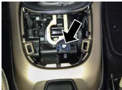
Gear Selector Override Access Hole
