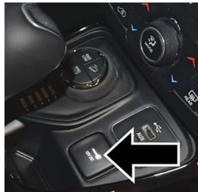
Front Power Outlet
