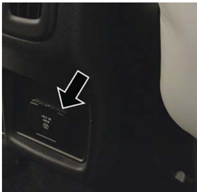
Power Inverter Location
