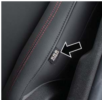
Front Supplemental Seat-Mounted Side Air Bag
