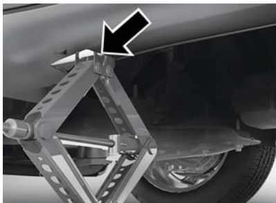
Front Jacking Location
