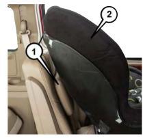
Car Seat With Head Restraint Folded
