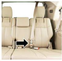
Mini-Latch And Buckle Connected
