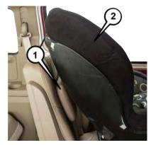
Car Seat With Head Restraint Folded
