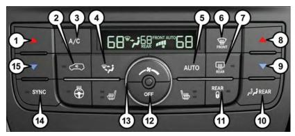
Three Zone Automatic Temperature Controls (ATC)
