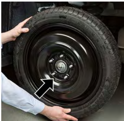
Installing Compact Spare
