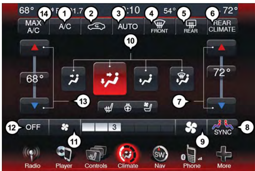
Radio 8.4 Automatic Climate Controls
