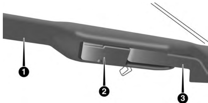
Wiper Blade With Release Tab In Locked Position
