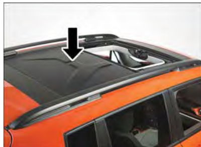
Installing Rear Panel
