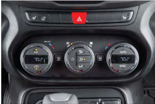
Automatic Temperature Controls (ATC)
