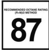
All available gasoline engines are designed to meet all emissions regulations and provide excellent fuel economy and performance when using high quality unleaded “regular” gasoline having a octane rating of 87 using the (R+M)/2 method. The use of premium gasoline is
