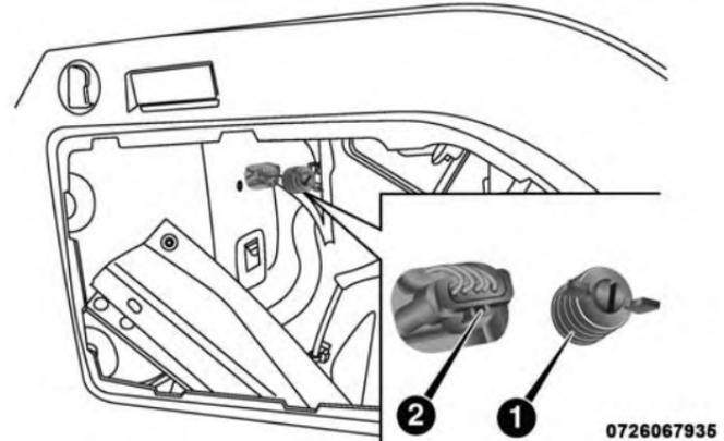
Rear Lamp Fastener and Electrical Connector
