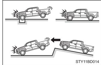
The SRS curtain shield airbags may also deploy under the situation shown in the illustration.
