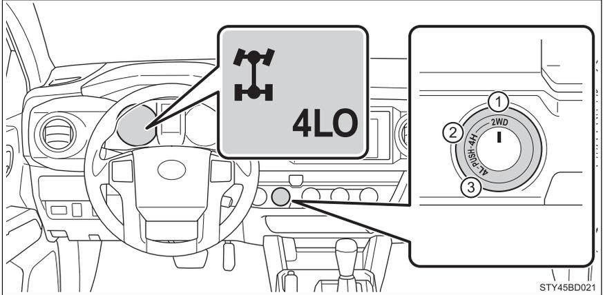
① "2WD" (high speed position, two-wheel drive)
