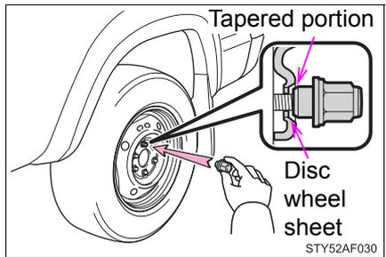
► Replacing an aluminum wheel with a spare aluminum wheel
