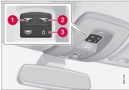
Light switches, front roof lighting
