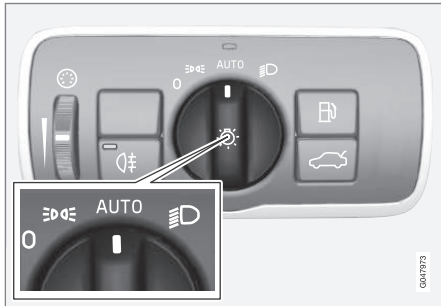
Headlight switch in the AUTO position
