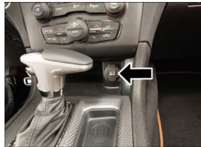
Front Power Outlet
