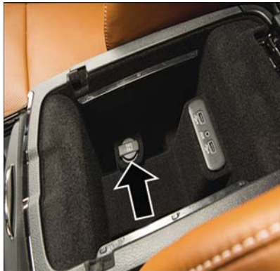
Center Console Power Outlet
