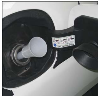
Emergency Fuel Filling Procedure
