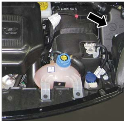
Front Distribution Unit
