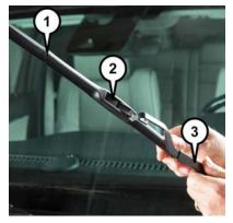
Wiper Blade Removed From Wiper Arm
