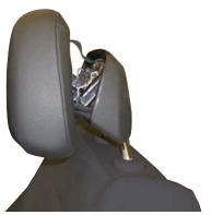
Active Head Restraint (AHR) Deployed
