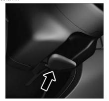
Manual Tilt/Telescoping Steering Column Handle
