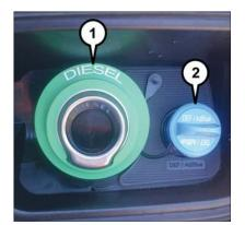
Fuel and Diesel Exhaust Fluid Fill Location
