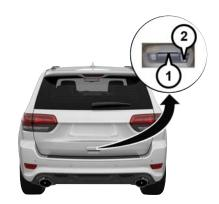
Electronic Liftgate Release/Liftgate **Passive Entry Location**
