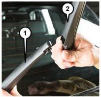
Wiper Blade Removed From Wiper Arm
