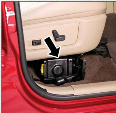
Jack And Tool Bracket Assembly
