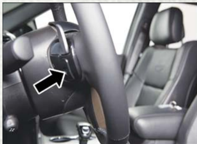
Steering Wheel Audio Controls
