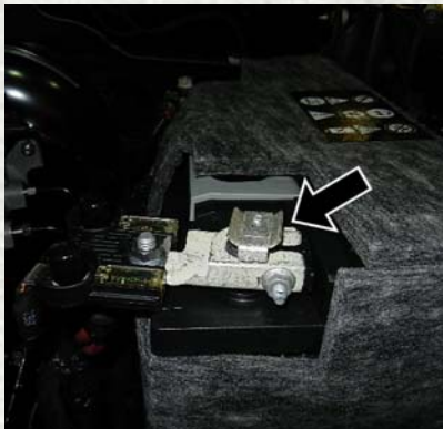
Positive Jumping Location
