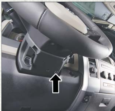
Shift Lock Manual Override Access Port
