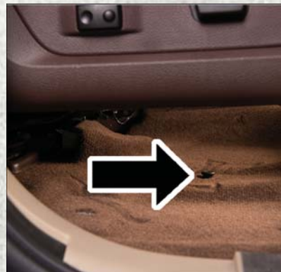
Floor Fastener Location
