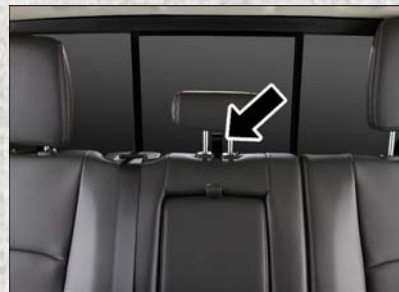
Crew Or Quad Cab Center Tether Anchorage With Head Restraint In Raised Position
