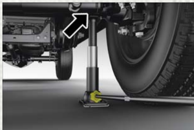
Front 4x2 Jacking Location
