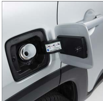
Fueling With Emergency Fuel Fill Funnel
