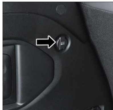
Rear Cargo Power Outlet
