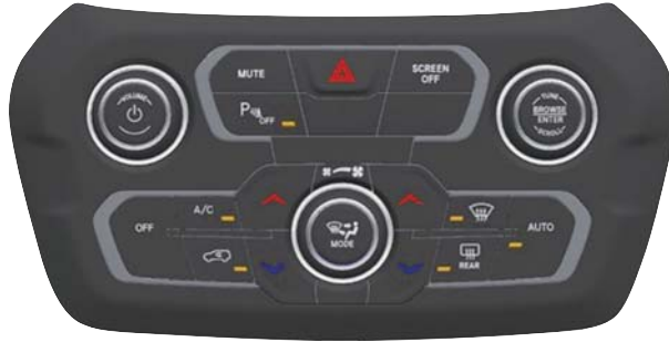
Automatic Temperature Controls (ATC)
