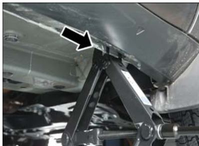
Front Jacking Location
