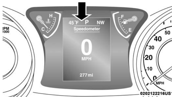
3.5 Inch Instrument Cluster Display Location
