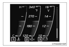
■ Engine coolant temperature gauge
