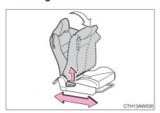
Lift the seatback angle adjustment lever.
