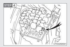
Remove the fuse with the pullout tool.
