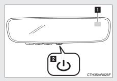
To turn the compass feature on/off, press and hold the () switch for more than 3 seconds or until the display turns on/off. The compass feature will default to on with each ignition cycle.
