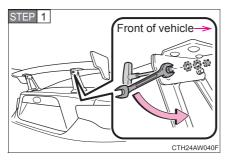
While holding the bolt on the rear side with a TORX wrench, using a wrench, socket wrench and socket, or similar tool, remove the nut and washers.
