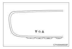
Within five seconds after programming a new HomeLink button, both of HomeLink's garage door status indicators will flash rapidly green indicating that the garage door two-way communication has been enabled. If your garage door status indicators flashed, two-way communication programming is complete.
