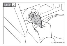
Touch the area behind the lock button and unlock button on the access key to the push-button ignition switch.
