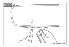
While the HomeLink indicator light is flashing orange, press and hold the hand-held remote button. Continue pressing the hand-held remote button until the HomeLink indicator light changes from orange to green. You may now release the hand-held remote button.
