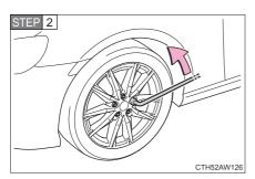
Slightly loosen the wheel nuts (one turn).
