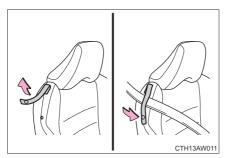
To enable the seatbelt to be easily extended, pass the seatbelt through the guide.
