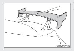
The rear wing can be adjusted to 2 different angles.
