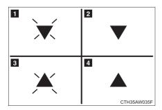
Recall and display (at any time) the last recorded garage door status message communicated to HomeLink by simultaneously pressing HomeLink buttons 1 and 2 for two seconds. HomeLink will display the last recorded status for three seconds.
