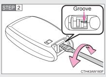
Insert the tip of a flathead screwdriver into the groove and remove the cover.
