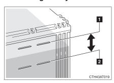
Check that the level is between "UPPER LEVEL" and "LOWER LEVEL".
