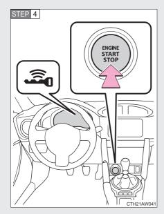
Press the push-button ignition switch shortly and firmly.
