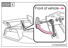
Install the bolt and washers. While holding the bolt with a TORX wrench, install the washers and nut and tighten the nut using a wrench, socket wrench and socket, or similar tool.
