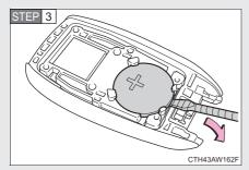
Remove the depleted battery.
