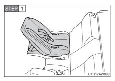
Place the child restraint system on the rear seat facing the rear of the vehicle.
