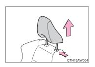
Pull the head restraint up while pressing the lock release button.
