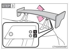
Adjust the angle of the rear wing.
