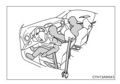
The pretensioner helps the seatbelt to quickly restrain the occupant by retracting the seatbelt when the vehicle is subjected to certain types of severe frontal or side collision or a vehicle rollover.
