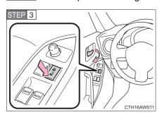
Open the driver's door while pressing and holding on the power door lock switch and continue to press for approximately 10 seconds after the driver's door has opened.
