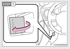
Pull the engine hood release lever.
