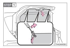
Remove the trunk lid panel cover clips and partly remove the trunk lid panel cover.
