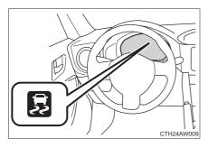
The slip indicator light will flash while the TRAC (brake LSD function)/Vehicle stability control (VSC) systems are operating.
