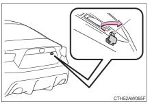
Turn the mechanical key clockwise to open.
