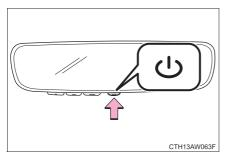
Press the U switch to turn the auto-dimming feature on/off. The auto-dimming feature is enabled when the switch's green LED indicator is on. The auto-dimming feature will default to on with each ignition cycle.
