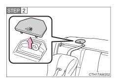
Remove the anchor bracket cover.
