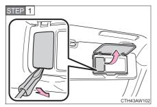
Open the cover and remove the lens.
