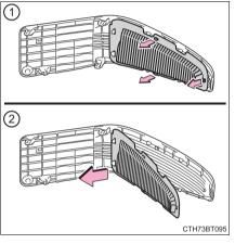
5 Remove the dust and clogs from the filter using a vacuum cleaner, etc.
