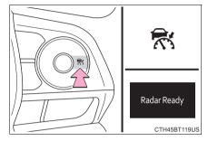
If the cruise control main switch is pressed and held for 1.5 seconds or more, the system turns on in constant speed control mode. ( $\rightarrow$ P. 279)
