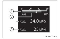
Displays the average vehicle speed since reset or elapsed time since reset, as selected in  $\bullet$ . ( $\rightarrow$ P. 105)
