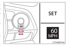
If the switch is operated while the vehicle speed is below approximately 30 mph (50 km/h) and a preceding vehicle is present, the set speed will be adjusted to approximately 30 mph (50 km/h).
