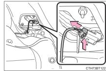
4 Turn the bulb base counter-clockwise.
