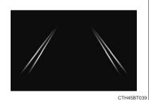
Indicates that the system is recognizing white (yellow) lines. When the vehicle departs from its lane, the white line displayed on the
