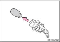
Install a new light bulb and then install the bulb base to the light unit by inserting it and turning it clockwise.
