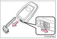
After using the mechanical key, store it in the electronic key. Carry the mechanical key together with the electronic key. If the electronic key battery is depleted or the entry function does not operate properly, you will need the mechanical key.  $(\rightarrow P. 509)$
