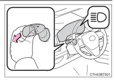
2 Press the Automatic High Beam switch.
