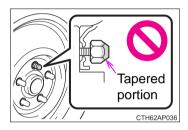
Never use oil or grease on the wheel bolts or wheel nuts. Oil and grease may cause the wheel nuts to be excessively tightened. leading to bolt or disc wheel damage. In addition, the oil or grease can cause the wheel nuts to loosen and the wheel may fall off, causing an accident and resulting in death or serious injury. Remove any oil or grease from the wheel bolts or wheel nuts.
