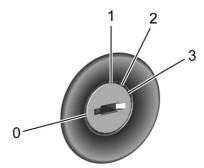
The ignition switch has four different positions.
