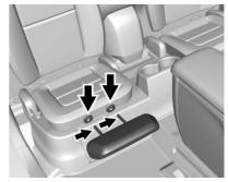
Insert the headrest posts into the holes on the front of the passenger side seat cushion to install the seat cushion extension. The notches on the posts should face the passenger side of the vehicle. Try to move the headrest to make sure it is locked in place.
