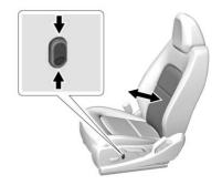
If equipped, press and hold the top of the control to increase lumbar support. Press and hold the bottom of the control to decrease lumbar support. Release the control when the desired level of support is reached.
