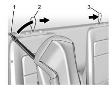
Route the top tether (1) through the loop (2) at the top of the seatback directly behind the child restraint and attach the top tether hook to the top tether loop at the top of the seatback for the opposite rear seating position (3).
