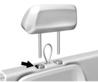
Press the button for the passenger side headrest at the top of the seatback and pull up.
