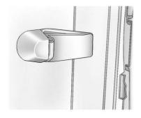
If the vehicle has this feature, squeeze the latch in the center of the window and slide the glass to open it.
