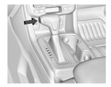
Range Selection Mode helps control the vehicle's transmission and vehicle speed while driving downhill or towing a trailer by letting you select a desired range of gears. To use this feature:
