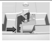
Go to the front of the vehicle to find the secondary hood release handle. The handle is under the front edge of the hood near the center. Push the handle to the right and at the same time raise the hood. To close the hood:
