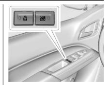
Press to activate the safety locks on the rear doors. The indicator light comes on when activated. The vehicle must be on, in ACC/ACCESSORY, or in Retained Accessory Power (RAP). See Retained Accessory Power (RAP).
