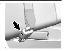
Disconnect the rear center seat belt latch from the mini-buckle by inserting the tip of the seat belt tongue into the slot on the buckle. Let the belt retract.
