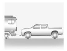
Only dinghy tow four-wheel-drive vehicles that have an N (Neutral) and a Four-Wheel Drive Low (4  $(\downarrow)$ ) setting.
