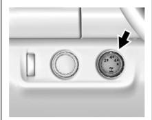
Use the transfer case knob, next to the steering wheel, to shift into and out of four-wheel drive for extra traction.
