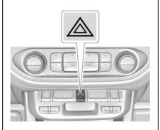
A: Press to make the front and rear turn signal lamps flash on and off. Press again to turn the flashers off.
