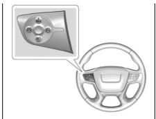
: Press to turn the system on or off. A white indicator comes on in the instrument cluster when cruise control is turned on.
