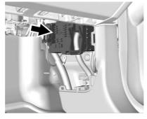
The instrument panel fuse block is behind the passenger side cowl side trim panel. Remove the plastic nut at the front of the cover, then pull the cover away from the trim panel to access the fuse block.
