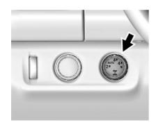
Use the transfer case knob next to the steering wheel to shift into and out of four-wheel drive.
