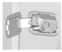
The hinged fuel door is on the driver side of the vehicle. To open the fuel door, push and release the rearward center edge of the door.
