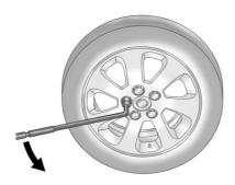
Use the wheel wrench and turn it counterclockwise to loosen the wheel nuts. Do not remove the wheel nuts yet.
