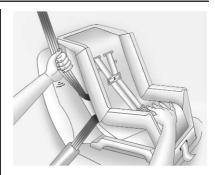
O. To tighten the belt, push down on the child restraint, pull the shoulder portion of the belt to tighten the lap portion of the belt, and feed the shoulder belt back into the retractor. When installing a forward-facing child restraint, it may be helpful to use your knee to push down on the child restraint as you tighten the belt.
