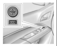
If equipped, adjust the power mirrors:
