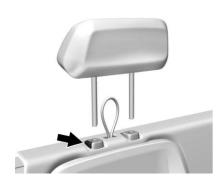
Press the button on the passenger side headrest and pull up.
