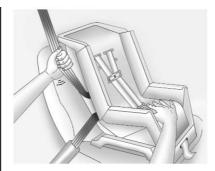
7. To tighten the belt, push down on the child restraint, pull the shoulder portion of the belt to tighten the lap portion of the belt, and feed the shoulder belt back into the retractor. When installing a forward-facing child restraint, it may be helpful to use your knee to push down on the child restraint as you tighten the belt.
