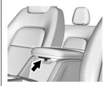
There is storage under the armrest in the center console. Press the button and lift. Depending on the options, there may be a USB port and/or auxiliary jack inside.
