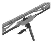
Press the release lever in the middle of the wiper blade where the wiper blade attaches.
