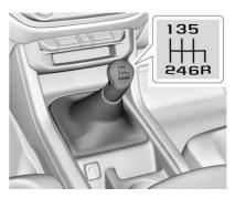
If equipped with a manual transmission, this is the shift pattern.
