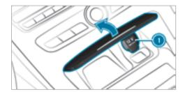
Lift up cap ① of the socket and insert the plug of the device.
