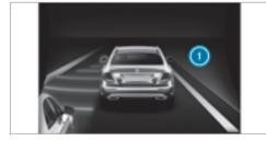
If a course-correcting brake application occurs, the red warning lamp flashes in the outside mirror and a warning tone sounds. In addition, display (1) indicating the danger of a side collision appears in the multifunction display.
