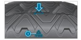
Six marks 1 show where the bar indicators (arrow) are integrated into the tire tread. They are visible once a tread depth of approximately  $\frac{1}{16}$  in (1.6 mm) has been reached.
