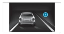
If a lane-correcting brake application occurs, display **(1)** appears in the multifunction display.
