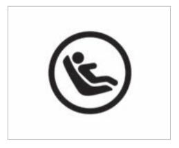
Symbol for fitting a LATCH-type (ISOFIX) child restraint system
