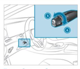
Reduce (5) or increase (6) the specified distance from the vehicle in front.
