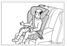
Check that the shoulder belt is correctly positioned over the child's shoulder and that the lap belt is as low as possible.  $(\rightarrow P. 31)$
