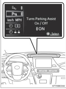
2 Each press of  $\odot$  of the meter control switches, changes ON and OFF. When ON is selected, the intuitive parking assist indicator turns on.
