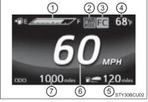
② ECO MODE indicator and POWER MODE indicator Displays the selected driving mode. (→P. 181)
