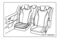
The surface of the seats with the side airbag is scratched, cracked, or otherwise damaged.
