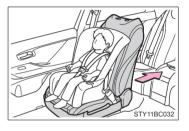
If the head restraint interferes with the child restraint system installation and the head restraint can be removed, remove the head restraint.
