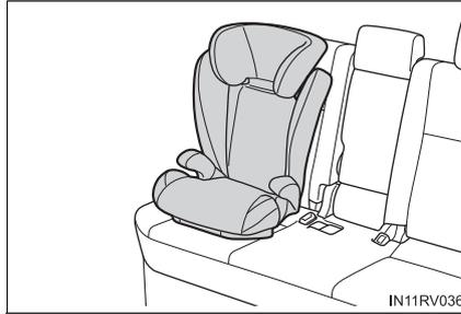
If your child restraint system interferes with a head restraint and cannot be installed properly, install the child restraint system after removing the head restraint. (→P. 152)
