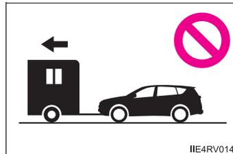
■ **To prevent causing serious damage to the hybrid transmission and AWD system**
