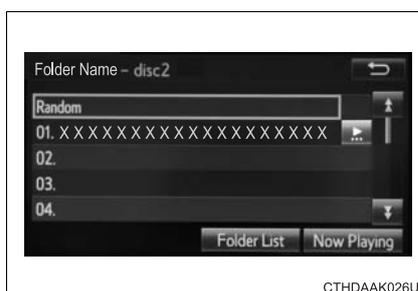
Turn the “TUNE•SCROLL” knob to move the cursor box to select a desired item from the list, and press the knob to play it. The track that is being played is highlighted.
