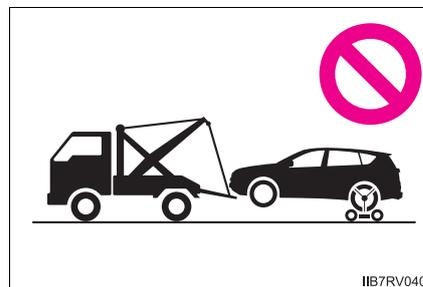
**Towing with a wheel-lift type truck**
