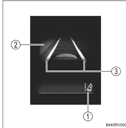
② Operation display of steering wheel operation support
