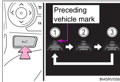
**Vehicle-to-vehicle distance settings (vehicle-to-vehicle distance control mode)**
