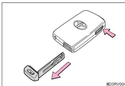
After using the mechanical key, store it in the electronic key. Carry the mechanical key together with the electronic key. If the electronic key battery is depleted or the entry function does not operate properly, you will need the mechanical key. (→P. 595)
