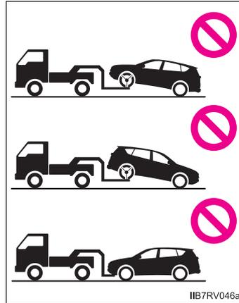
■ **While towing (vehicles with a towing eyelet)**
