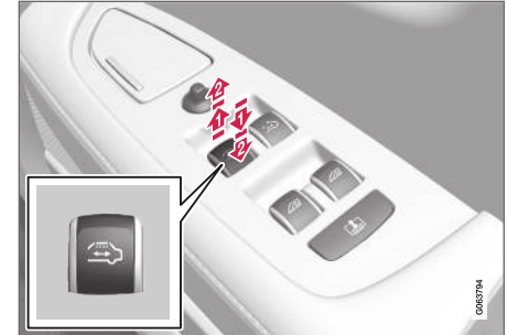
Sun curtain control.
