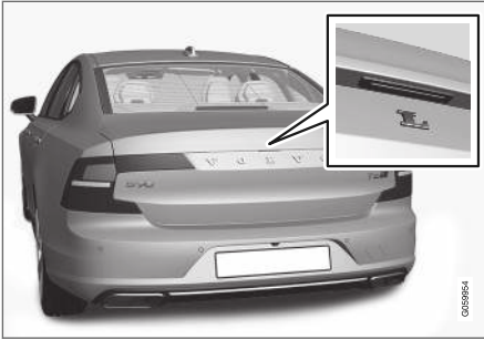
Rubberized pressure plate on the trunk lid used only for unlocking.
