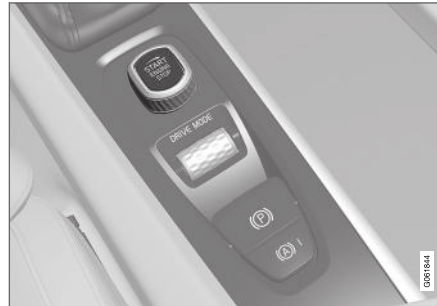
Start knob in the tunnel console.
