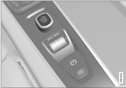
Start knob in the tunnel console.
