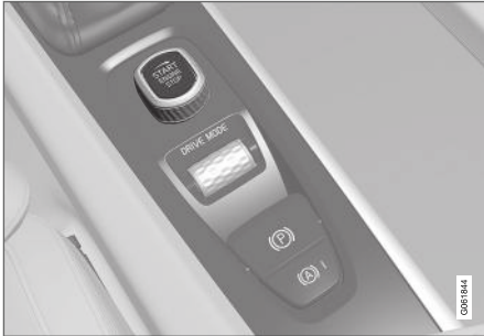
Start knob in the tunnel console.
