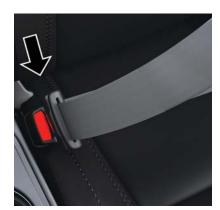
**Inserting Latch Plate Into Buckle**
