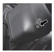
Power Tilt/Telescoping Steering Control
