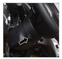
Power Tilt/Telescoping Steering Control Location
