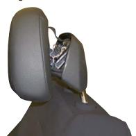
Active Head Restraint (AHR) Deployed
