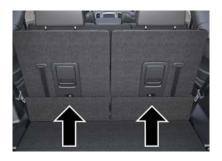
Pulling Down The Carpet Floor Panel To Access Top Tether Strap Anchorage
