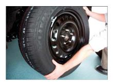
Installing Spare Wheel/Tire
