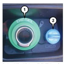
Fuel and Diesel Exhaust Fluid Fill Location
