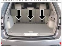
Top Tether Strap Anchorage (Located On Seatback)
