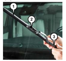
Wiper Blade Removed From Wiper Arm
