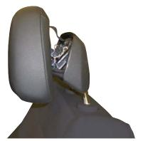
Active Head Restraint (AHR) Deployed
