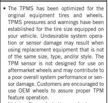
Using aftermarket tire sealants may cause the Tire Pressure Monitoring System (TPMS) sensor to become inoperable. After using an aftermarket tire sealant it is recommended that you take your vehicle to an authorized dealership to have your sensor function checked.
