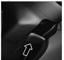
Manual Tilt/Telescoping Steering Column Handle
