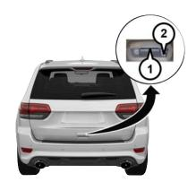
Electronic Liftgate Release/Liftgate **Passive Entry Location**
