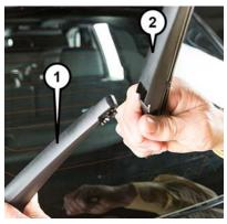
Wiper Blade Removed From Wiper Arm
