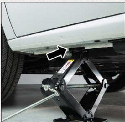
Front Jacking Location Engaged
