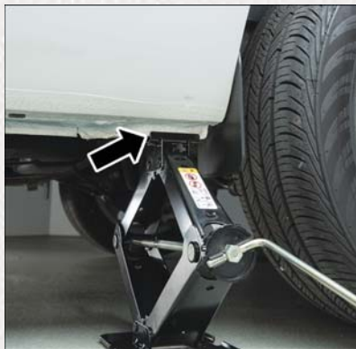
Rear Jacking Location Engaged
