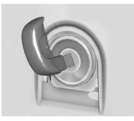
Remove any additional items attached to the key — such as keys, rings, or tags — then fully insert the key into the manual release.
