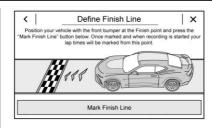
To set the finish line, position the vehicle with the front bumper at the start/finish point. From the PDR menu, touch Define Finish Line and then touch Mark Finish Line. This can be done with the vehicle moving.
