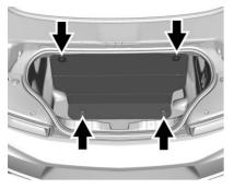
The trunk partition can be attached or detached to upper trunk brackets. With the convertible top up, the trunk partition can be unsnapped and laid flat.
