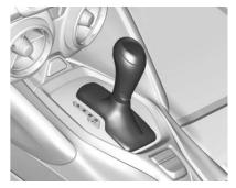
DSC allows shifting an automatic transmission similar to a manual transmission. To use the DSC feature:
