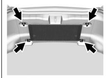
For vehicles with a convenience net inside the trunk, it can be used to secure loose items.
