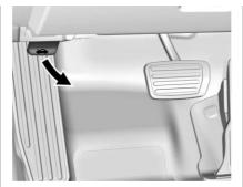
1. Pull the release handle below the instrument panel to the left of the steering wheel and forward of the foot rest.
