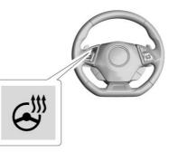
If equipped, press to turn the heated steering wheel on or off.
