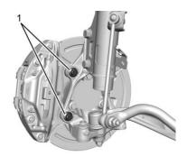
Apply liquid thread adhesive to the caliper bolts (GM Part No. 9985399 – Loctite 272 –
