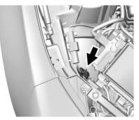
The electrical cord is on the passenger side of the engine compartment, next to the engine compartment fuse block.
