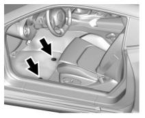
The driver side floor mat is held in place by two hook-type retainers.
