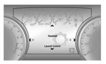
Ensure the parking brake is disengaged to re-enter Launch Control.
