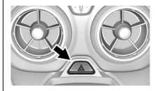
A: Press to make the front and rear turn signal lamps flash on and off. This warns others that you are having trouble. Press again to turn the flashers off.
