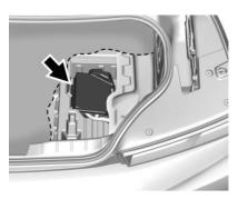
The rear compartment fuse block is on the right side under the trunk load floor.
