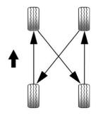
Use this rotation pattern when rotating tires of the same size installed on all four wheel positions.
