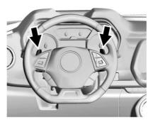
Tap Shift allows you to manually control the automatic transmission. To use Tap Shift, the shift lever must be in DSC mode. Vehicles with this feature have indicators on the steering wheel. The paddles are on the back of the steering wheel. Tap the left paddle (-) to downshift, and the right paddle (+) to upshift. The Driver Information Center (DIC) display indicates the gear the vehicle is in.
