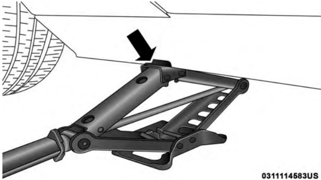
Front Jacking Location
