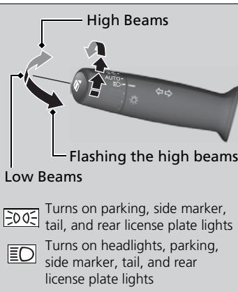
Rotating the light switch turns the lights on and off, regardless of the power mode setting.
