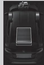
Shows the engine and High Voltage battery power flow, indicating what is supplying power to the vehicle and/or charging the battery.
