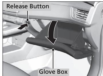
Press the release button to open the glove box.
