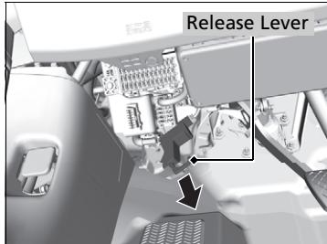
1. Pull the release lever under the lower left corner of the dashboard.
