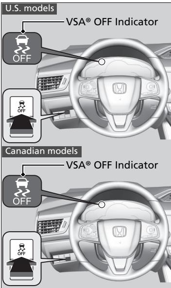
This button is on the driver side control panel. To partially disable VSA® functionality/features, press and hold it until you hear a beep.
