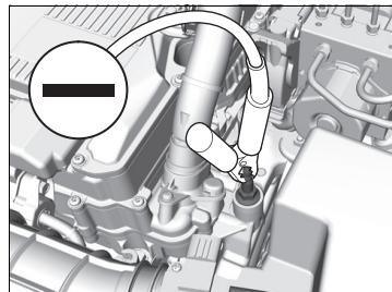
5. Connect the other end of the second jumper cable to the power system mounting bolt as shown. Do not connect this jumper cable to any other part of the vehicle.
