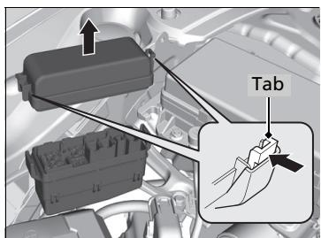
Fuse locations are shown on the fuse box cover. Locate the fuse in question by the fuse number and box cover number.
