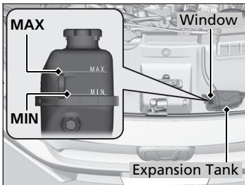
1. Check the fluid level in the tank from the window.
