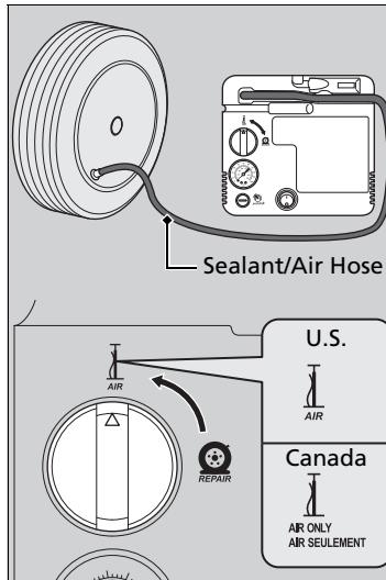
4. Recheck the air pressure using the sealant/air hose on the compressor.
