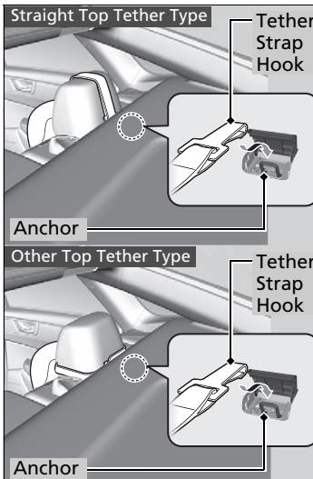
3. Open the tether anchor cover behind the head restraint.
