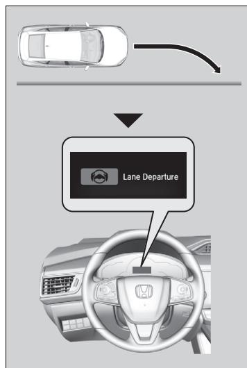
The front camera behind the rearview mirror monitors left and right lane markings (in white or yellow). If your vehicle is getting too close to detected lane markings without a turn signal activated, the system, in addition to a visual alert, applies steering torque and alerts you with rapid vibrations on the steering wheel, to help you remain within the detected lane.
