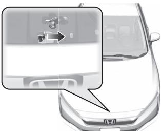
3 When finished, close the hood and make sure it is firmly locked in place.
