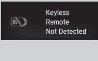
Warning buzzers may sound from inside and/or outside the vehicle to remind you that the smart entry remote is out of the vehicle. If the buzzer continues even after the remote is put back inside, place it to be within its operational range.
