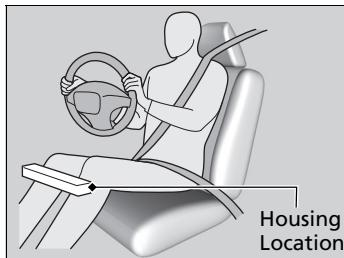
The driver's knee airbag is housed under the steering column.
