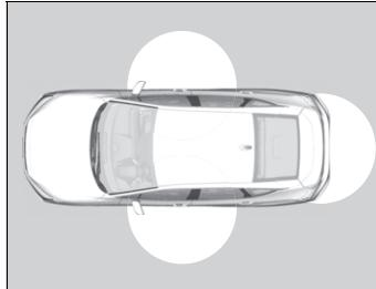
When you carry the smart entry remote, you can lock/unlock the doors and open the trunk. You can lock/unlock the doors within a radius of about 32 inches (80 cm) of the outside door handle or trunk release button.
