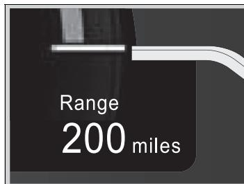
Shows the estimated distance you can travel on the remaining power and fuel. This estimate is based on the fuel economy and energy consumption of your previous trips and the remaining high voltage battery charge level.
