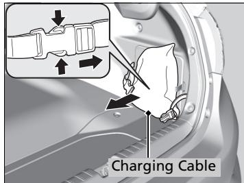
1. Remove the charging cable by releasing the belt.
