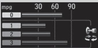
Shows the average fuel economy for the last three driving cycles (1 – 3), and the current driving cycle (0) in mpg or l/100 km.
