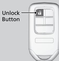
**To open:** Press the unlock button, and then within 10 seconds, press it again and hold it.
