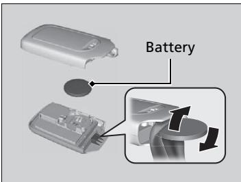
Replacing the Button Battery
