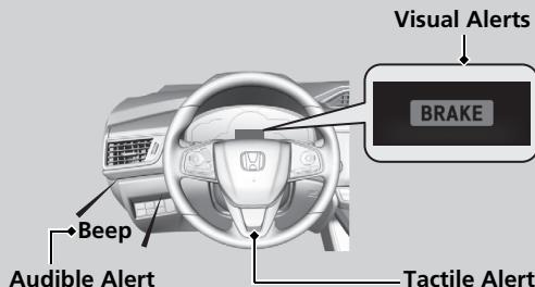
At system's earliest collision alert stage, you can change the distance (**Long/Normal/Short**) between vehicles at which alerts will come on through audio/information screen setting options.
