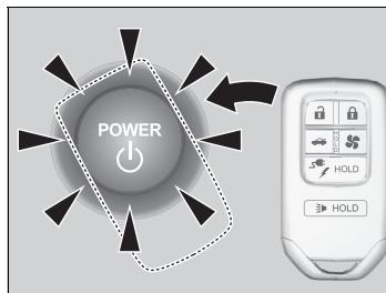
1. Touch the center of the **POWER** button with the **H** logo on the smart entry remote while the indicator on the **POWER** button is flashing. The buttons on the smart entry remote should be facing you.
