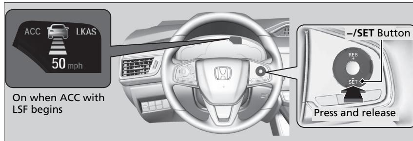
**When driving at about 25 mph (40 km/h) or above:** Take your foot off the pedal and press the **-/SET** button when you reach the desired speed. The moment you release the button, the set speed is fixed, and ACC with LSF begins.
