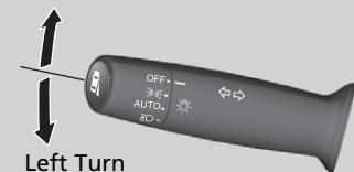
The turn signals can be used when the power mode is in ON.
