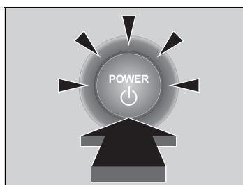
2. Depress the brake pedal and press the **POWER** button within 10 seconds after the beeper sounds and the **POWER** button changes from flashing to on.
