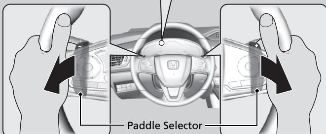
Increase the deceleration stage when pulling the **-** paddle selector (left side)
