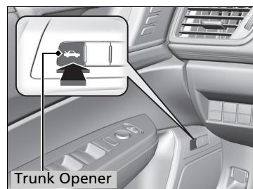
Pressing the trunk opener on the driver's door unlocks and opens the trunk.
