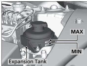
1. Check the fluid level in the tank.
