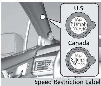
1. Apply the speed restriction label to the location as shown.
