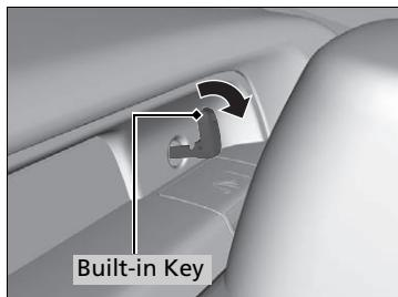
1. Insert the built-in key into the cylinder and turn the key clockwise (as shown).
