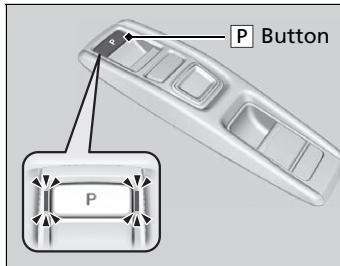
The gear position changes to **P** when you press the **P** button while the vehicle is parked with the power mode in ON. The indicators on the sides of the **P** button come on.
