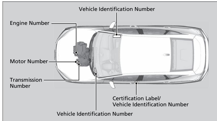
Vehicle Identification Number (VIN), Engine Number, Motor Number, and Transmission Number
