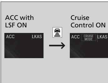
Press and hold the
