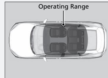
You can start the power system when the smart entry remote is inside the vehicle.
