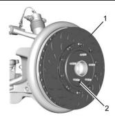
Install the rotor (1) with the fastener (2). Torque to 10 N•m (89 lb inch).
