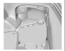
The tow eye can be stowed in the vehicle in the passenger side trunk area, below the carpet.
