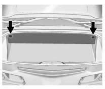
Pull the divider up and snap it into place on both sides of the trunk.
