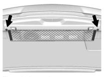
The vehicle may have a convenience net to be used for small loads. Attach the net to the hooks on the rear of the storage area. The net should not be used to store heavy loads.
