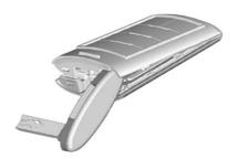
Use the oval base of the key blade to separate the two halves of the transmitter.
