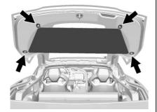
Attach the elastic loops on the four corners of the cargo cover to the hooks on the front and rear corners of the hatch.
