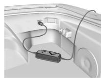
Some vehicles have a battery maintainer package. Follow the instructions provided with the battery maintainer package to keep the battery charged when the vehicle is not in use. Plug the battery maintainer into the rear
