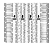
Treadwear indicators are one way to tell when it is time for new tires. Treadwear indicators appear when the tires have only 1.6 mm (1/16 in) or less of tread remaining. See *Tire Inspection*  $\Rightarrow$  278 and *Tire Rotation*  $\Rightarrow$  279.
