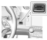
The vehicle has an electronic keyless ignition with pushbutton start.
