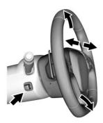
Press the control to move the tilt and telescoping steering wheel up and down or forward and rearward. Both the tilt and telescoping steering column positions can be stored with your memory settings, if equipped. See *Memory Seats* ⇒ 60.
