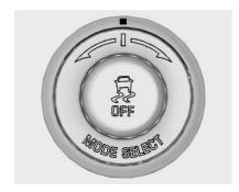
The Driver Mode Selector knob is on the console behind the shift lever.
