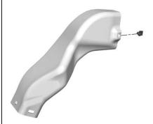
2. Position the u-nut on the upper duct.
