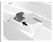
Insert the front of the roof panel so that the indents lay on top of the receivers.
