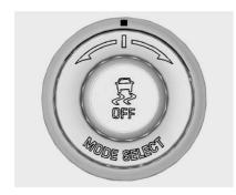
In order to select this optional handling mode, the vehicle mode must be in Sport or Track Mode. In vehicles equipped with Performance Traction Management (PTM), the Competitive Driving Mode is only available in Sport Mode. In vehicles not equipped with PTM, the Competitive Driving Mode is available in Sport and Track Mode. Then quickly press on the center console two times. STABILITRAK/ESC COMPETITIVE MODE displays in the Driver Information Center (DIC).
