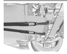
The vehicle is also equipped with secondary attachment points to be used to pull the vehicle onto a flatbed car carrier from a flat road surface. Do not use these attachment points to pull the vehicle from snow, mud, or sand.
