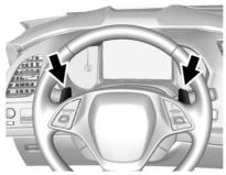
When the shift lever is moved to M (Manual Mode), the transmission enters Manual Mode. The transmission will hold the current gear until a change is requested. The paddles on the steering wheel can be used to manually upshift or downshift the transmission. The right (+) plus paddle upshifts, and the left (-) minus paddle downshifts.
