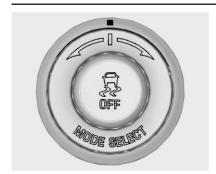
The PTM system contains five modes. These modes are selected by turning the Selective Ride Control/Performance Traction Management MODE SELECT knob on the center console. Scroll up or down through modes 1–5 by turning the MODE SELECT knob to the right or left.
