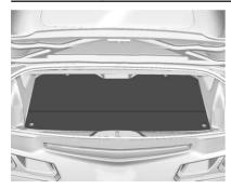
With the convertible top up, the trunk partition can be unsnapped and laid flat to increase trunk cargo space.
