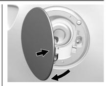
To open the fuel door, push and release the rearward center edge of the door. The fuel door is locked when the vehicle doors are locked. Press on the RKE transmitter to
