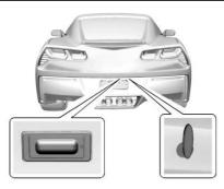
Press the hatch/trunk release touch pad with the RKE transmitter within range or use the key in the key cylinder. See Remote Keyless Entry (RKE) System ⇒ 26 and Keys ⇒ 25.
