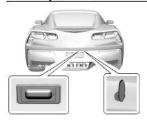
Press the hatch/trunk release touch pad with the RKE transmitter within range or use the key in the key cylinder. See Keys \$\dip\$ 25.
