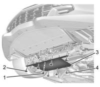
Remove the four front (2) and three rear (4) front compartment air deflector screws.
