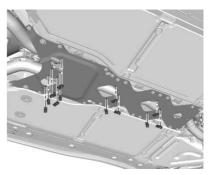
Install the 12 U-nuts onto the tunnel brace. Align the threaded holes in the U-nuts with the holes in the tunnel brace.
