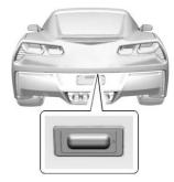
Press the hatch/trunk release touch pad to open the trunk if the RKE transmitter is within 1 m (3 ft).
