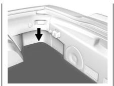
Open the hatch/trunk and lift the carpet on the passenger side of the vehicle to gain access to the battery cover.
