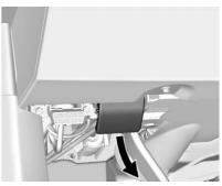
Pull the hood release lever inside the vehicle. It is below the instrument panel on the driver side.
