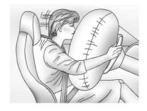
The driver frontal airbag is in the center of the steering wheel.
