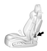
If equipped, lift the latch to fold a seatback forward.
