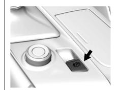
The vehicle has an Electric Parking Brake (EPB). The EPB can always be activated, even if the ignition is off. To prevent draining the battery, avoid repeated cycles of the EPB system when the engine is not runnina.
