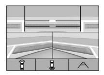
If equipped, a view of the area in front of the vehicle displays in the infotainment display. The display shows a front, top down view at the top and left and right front camera images on the bottom.
