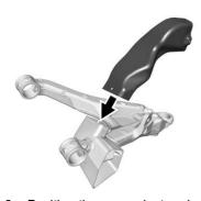
Position the upper duct and snap it into the tabs on the airbox assembly. Position the upper duct through the bottom of the vehicle to bring it close to the tab position.
