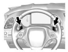
The Manual Paddle Shift system can be used in D (Drive) or M (Manual Mode). The system is activated by pressing the left paddle to downshift and the right paddle to upshift. The current gear will be displayed in the instrument cluster, or the Head-Up Display (HUD), if equipped.
