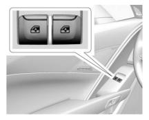
The power windows work when the ignition is on, in ACC/ACCESSORY, or when Retained Accessory Power (RAP) is active. See Retained Accessory Power (RAP) ⇒ 183.
