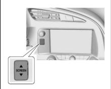
Press ▲ SCREEN and hold to open and access the storage behind it.
