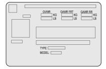
A vehicle-specific Certification label is attached to the rear edge of the driver door. It may show the gross weight capacity of the vehicle, called the Gross Vehicle Weight Rating (GVWR). The GVWR includes the weight of the vehicle, all occupants, fuel and cargo.
