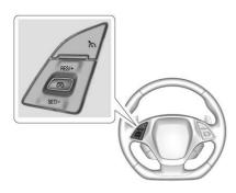
harmonic Press to turn cruise control on or off. A white indicator comes on in the instrument cluster when cruise is turned on.
