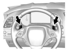
The system is activated and deactivated by pressing either of the paddles marked REV MATCH on the steering wheel. The system
