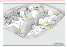
The pretensioners do not activate in the event of a minor frontal impact, a minor side impact or a rear impact.
