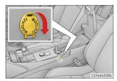
The power outlet can be used when the engine switch is in ACCESSORY or IGNITION  $\mbox{ON}$  mode.
