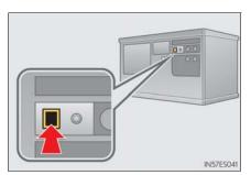
Press and hold the desired HomeLink® button (inside the vehicle) for 2 seconds and release it. Repeat this sequence (press/hold/release) up to 3 times to complete programming. If the garage door opener motor operates when the HomeLink® button is pressed, the garage door opener motor recognizes
