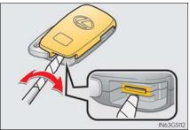
**3** Remove the depleted battery.
