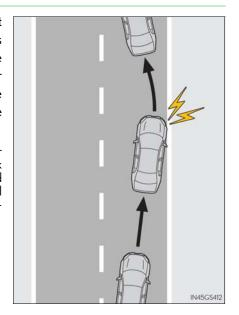
When the system determines that the vehicle might depart from its lane, the system provides assistance as necessary by operating the steering wheel in small amounts for a short period of time to keep the vehicle in its lane.
