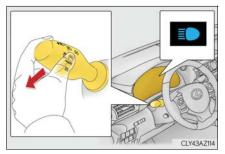
**2** Press the Automatic High Beam switch.
