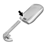
Press the button on the back of the RKE transmitter to pull out the key. Never pull the key out without pressing the button.
