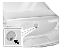
Press the bottom of the emblem above the license plate when all doors are unlocked or when the transmitter is within 1 m (3 ft) of the rear of the vehicle.
