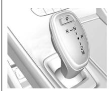
The shift pattern is displayed in the top of the shift lever. The selected gear position will illuminate red on the shift lever, while all others will be displayed in white. If the shift is not immediate, as in very cold conditions, the indicator on the shift lever may blink until it is fully engaged.
