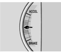
This gauge is a guide to driving in an efficient manner and will vary based on driver input. To maximize efficiency, keep the leaf in the solid green zone in the center of the gauge. The leaf moves down when braking and up when accelerating. When either is done aggressively. the vehicle is being driven less efficiently and the gauge will move further from the center.
