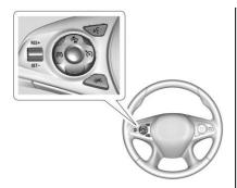
(iii): Press to turn the system on or off. The indicator turns white on the instrument cluster when ACC is turned on.
