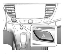
: Press to make the front and rear turn signal lamps flash on and off. Press again to turn the flashers off.
