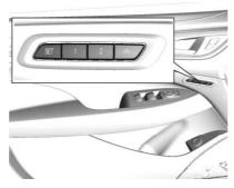
If equipped, memory seats allow two drivers to save and recall their unique seat positions for driving the vehicle, and a shared exit position for getting out of the vehicle. Other feature positions may also be saved, such as power mirrors and power steering wheel, if equipped.
