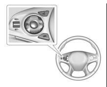
(iii): Press to turn cruise control on or off. A white indicator comes on in the instrument cluster.
