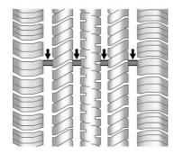
Treadwear indicators are one way to tell when it is time for new tires. Treadwear indicators appear when the tires have only 1.6 mm (1/16 in) or less of tread remaining. See *Tire Inspection* ⇒ 282 and *Tire Rotation* ⇒ 283.
