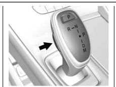
This vehicle is equipped with an electronic transmission. The shift lock release button is designed to prevent shifting out of P (Park), unless the ignition is on, the brake pedal is applied, and the shift lock release button is pressed.
