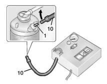
Attach the air only hose (10) to the sealant canister inlet valve (1) by turning it clockwise until tight.
