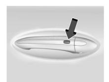
Press the lock/unlock button when the RKE transmitter is within 1 m (3 ft) of the driver door handle. When unlocking from the driver door, the first press unlocks that door; press again within five seconds to unlock all passenger doors. See *Remote Keyless Entry* (*RKE*) *System Operation* ⇒ 30.
