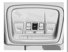
If equipped, the rear window sunshade switch is on the overhead console. To open the sunshade, press and release the switch. The sunshade will fully extend. To close the sunshade, press and release the switch again. The sunshade will fully close.
