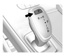
Press the P button on the shift lever.
