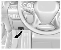
Pull the interior hood release handle located to the left of the steering column below the instrument panel.
