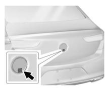
Press the bottom of the emblem above the license plate when all doors are unlocked.
