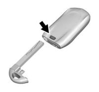
Press the button on back of the RKE transmitter to pull out the key. Never pull the key out without pressing the button.
