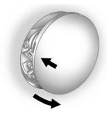
To open the fuel door, push and release the rearward center edge of the door.
