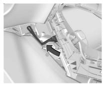
Pull the manual park release lever 90° to its latching position.
