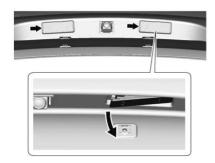
Push the lamp assembly toward the center of the vehicle, then move the lamp downward, and remove it from the vehicle body.
