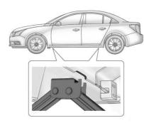
Position the jack lift head at the jack location nearest the flat tire. The location is indicated by a notch in the vertical bottom edge of the body side sheet metal.
