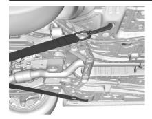
The vehicle is equipped with specific attachment points to be used by the towing provider. These holes may be used to pull the vehicle from a flat road surface onto the flatbed tow truck.
