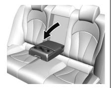
The rear seat has an armrest in the center of the seatback. Lower the armrest to access the two cupholders and the storage area.
