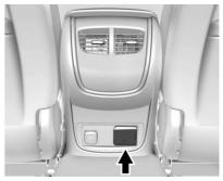
The vehicle may have a power outlet that can be used to plug in electrical equipment with a maximum limit of 150 watts.
