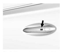
The RKE transmitter must be within 1 m (3 ft) of the door being opened.
