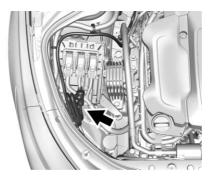
The electrical cord is on the driver side of the engine compartment, between the fender and the engine compartment fuse block.
