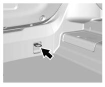
The vehicle has two cargo tie-downs in the rear compartment.
