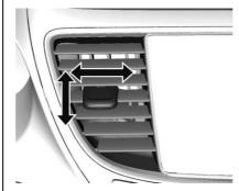
Use the slider knob on the air vent louvers to change the amount and direction of the airflow.
